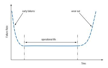
Estimated field failure rate: ≤ 0.15 ppm (failures per year/produced number of capacitors per year)
