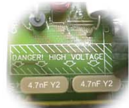
Photo showing keepout zone which may be eliminated with Evox Rifa Y capacitors.
